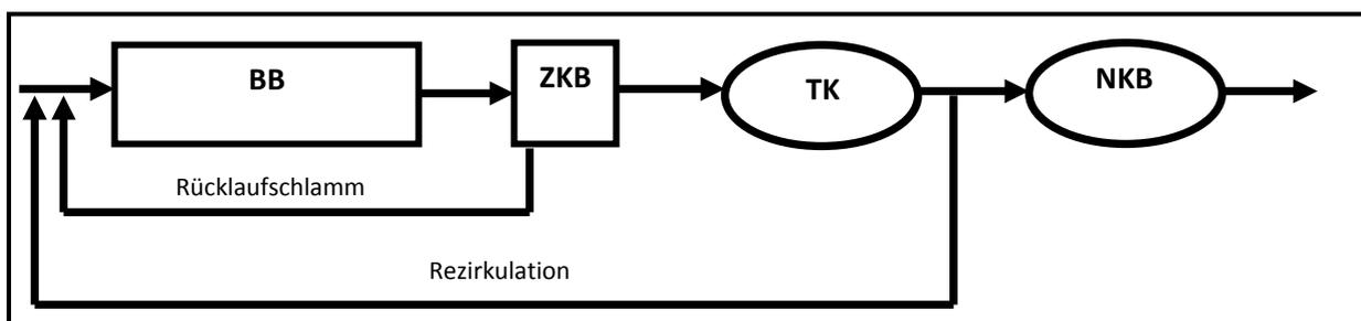
Fig. 1: Activated sludge process with upstream denitrification and downstream nitrogen-fixing trickling filter
