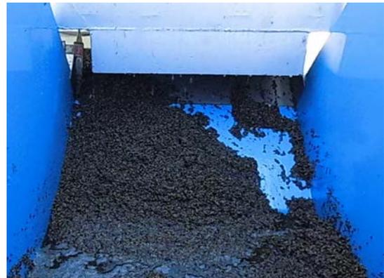
Fig. 4: Separated snail shells in the discharge of the RoMesh® trial plant
